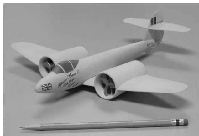
**Matt Keennon** flies his new Peanut scale Gloster Meteor which is modeled after the air speed record setting plane of 1945. It's a twin EDF (electric ducted fan) model that flies very fast, but manage to do a circle in a gym hall.
