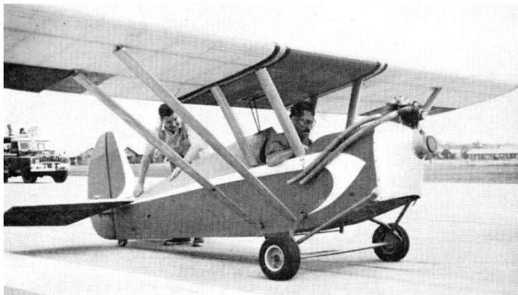
Flight Lieutenant Ray Lawrence runs the Triumph M/Cycle engine in his "Kuching Special" made while stationed in Borneo. Direct drive at 3 400 r.p.m. is a disadvantage, leading to poor airscrew efficiency. Weighing only 335 lbs. less pilot, the "Special" hopped a few times before enforced dismantling due to Service posting.
